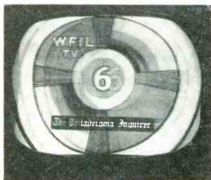
Fig. 1 — Ghost image on black and white screen. On color tube this image will be slightly more noticeable to observer.
