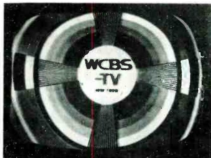
Fig. 3 — Interlace pattern appearing on black and white screen. Loss of interlace on color screen will result in a coarse horizontal line structure and degradation of pix.
